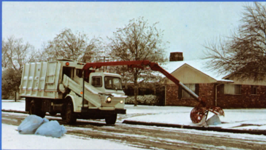
The MBR at work: garbage from the left side of the street...
