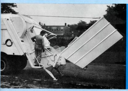
Cable mechanism lifts, tilts and empties Roto-Pac Container in seconds. No piles of rubbish to clean up.
